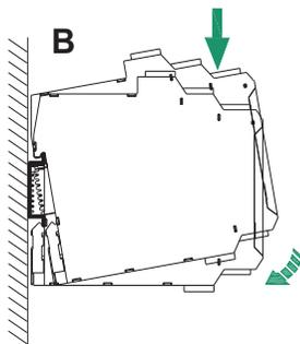
B. Snap metal lock onto mounting rail, then rotate the apparatus, as figure B, press down the apparatus onto mounting rail, make sure that the BUS connector pins of apparatus and BUS socket are in close contact.
