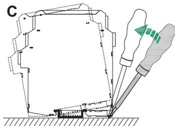
C. Pry the metal lock off the rail with screwdriver as arrow shown, pull downward the springs, and rotate the apparatus.
