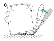
C. Pry the metal lock off the rail with screwdriver as arrow shown, pull downward the springs, and rotate the devices.
