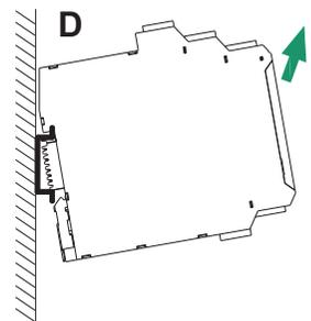
D. Remove the apparatus as arrow shows.
