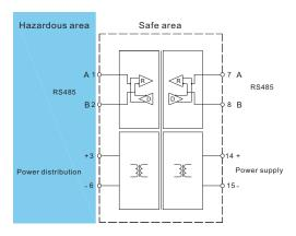
O The transmission cable in the figure is recommended to use the shielded twisted pair.
