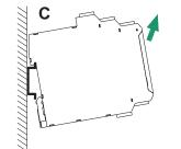
C. Remove the safety barrier as arrow shows.O As far as possible to mount it vertically, In order to dissipation the heat of the apparatus.
