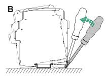
B. Pry the metal lock off the rail with screwdriver as arrow shown, pull downward the springs, and rotate the safety barrier.
