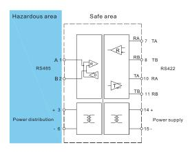
O The transmission cable in the figure is recommended to use the shielded twisted pair.
