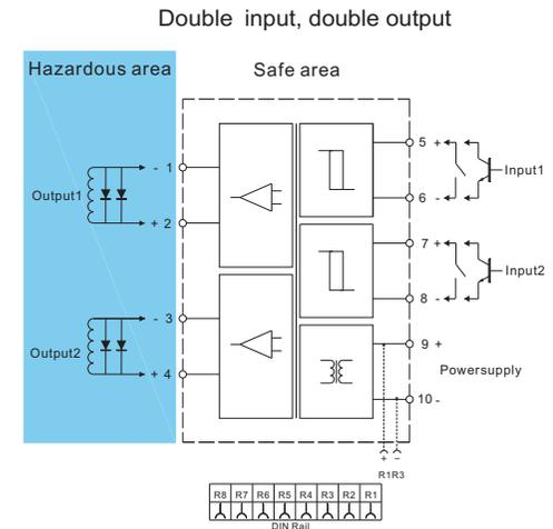
○ DIN rail power supply function is selectable at ordering.
